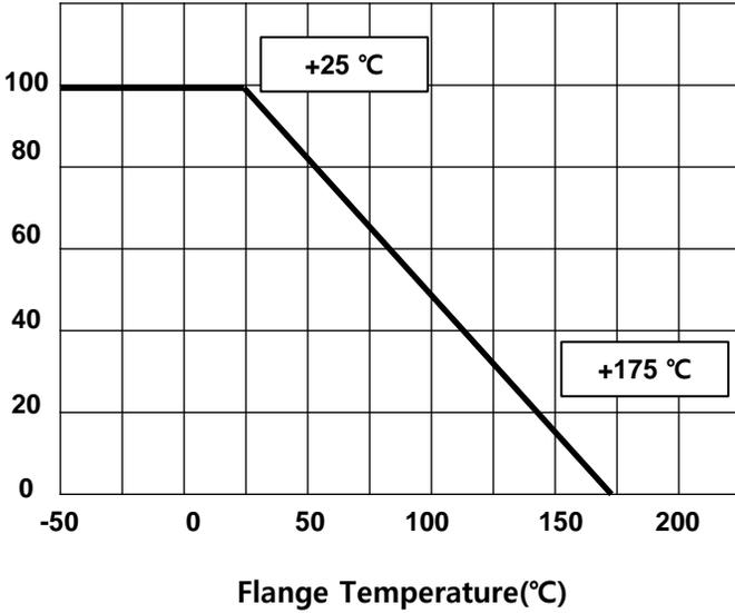
The TF223 Series Thick Film Resistors must be attached to a suitable heat sink. Without a heat sink the maximum power rating is 1 W. The maximum internal resistor temperature is 175 °C.
